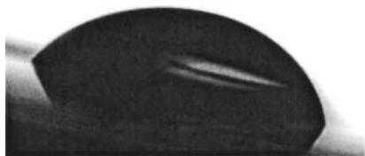
FIG. 3. Image of an EG drop on a solid surface tilted close to its critical inclination. The drop volume is 13.4 mm 3 and the inclination is 12°.
