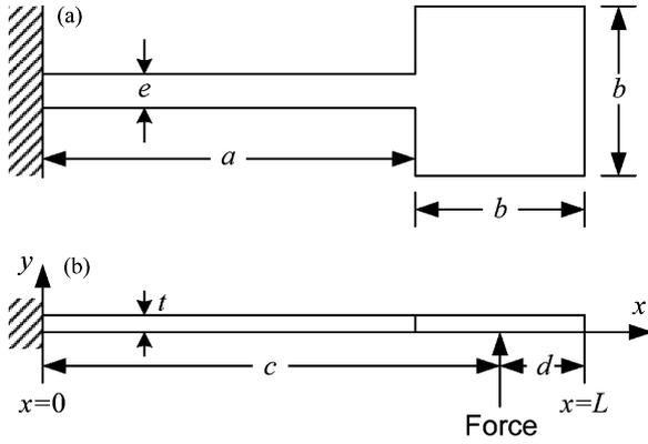
Fig. 1. Shape and dimension of a cantilever beam. (a) Top view. (b) Side view.
