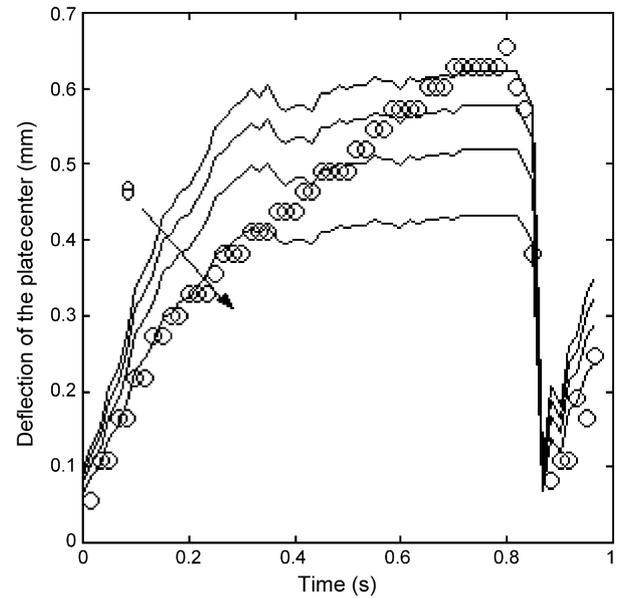
Fig. 5. Comparison of the experimental results (circles) with the theoretical predictions (solid lines). For theoretical predictions, we used different values of  $\theta$ , and  $\theta$  increases in the direction of the arrow taking the values  $0^\circ$ ,  $30^\circ$ ,  $45^\circ$ , and  $60^\circ$ .
