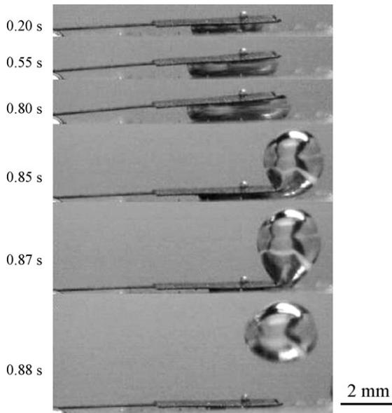
Fig. 2. Sequential images of a growing vapor bubble and a deforming cantilever beam.
