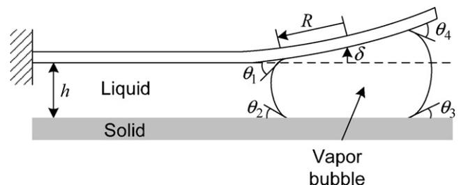
Fig. 3. A schematic of the deflected beam due to a growing bubble.
