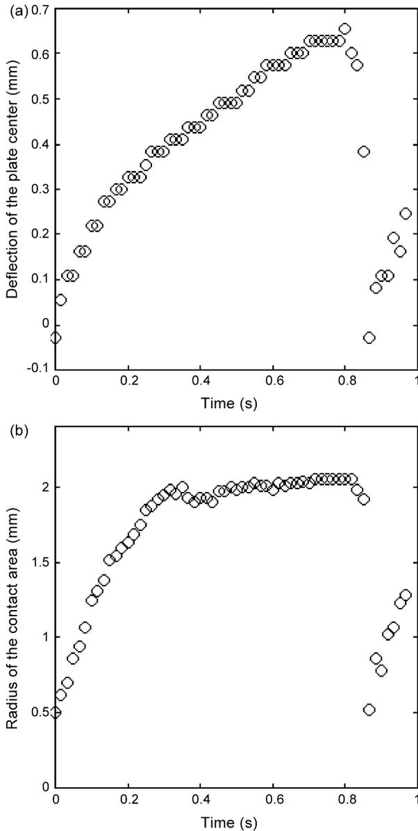
Fig. 4. Measurement results for the temporal evolution of (a) the deflection of the plate center and (b) the radius of the bubble/plate contact area.
